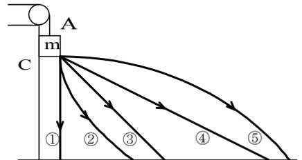
(解答)(1)  $A$ :  $ma = mg - T$  ,  $B$ :  $3ma = T - \frac{3}{5}mg$  (2)  $a = \frac{g}{10}$  ,  $T = \frac{9}{10}mg$  (3)  $\frac{3g}{10}$
